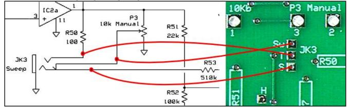
• Use a switching type jack for the manual sweep input jack (JK3). Something similar to Mouser pn 568-NYS218 should work well. The jack sleeve should be grounded, so the jack does not need to be isolated from the enclosure.
