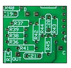
The value of the mixing resistors at the output buffer (R41, R42) has been reduced to allow higher than unity volume at the output, and a 10K output volume pot can be added as shown in the schematic, above. If a panel mounted volume control is not desired, a 10K trim pot can be installed in the perfboard area in the lower left corner of the PCB and connected to the circuit output with a flying lead to provide an internal level setting for the output volume.
