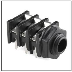
This type of jack has two contacts each for the sleeve, ring and tip connections. On one side of the jack (as shown above) each contact has a normally closed switch. When a plug is inserted, the switches are all opened. See schematic and wiring diagram for wiring details. The CV pedal that you use for Rate control should have a cord with a stereo plug. I tried a couple different pedals, one with a 100k pot and one with a 20k pot, and both seemed to work reasonably well.
